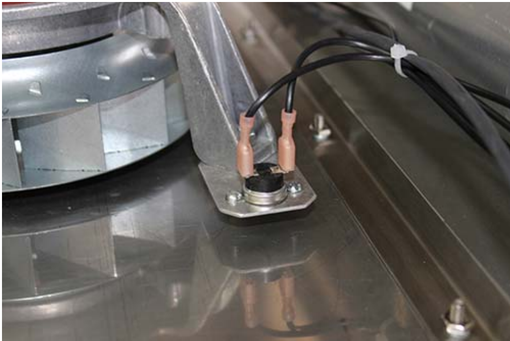
Top Oven Compartment Thermostat set to 145°F
